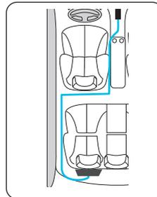
Route the cable under carpets or other plastic details between the control knob and the unit. To avoid cable damage when adjusting car seats, do not route the cable too close to the seat tracks. Coil any cable excess and fasten with the supplied cable tie.
