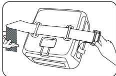
Thread the mounting strap through the unit as shown. Velcro side faces unit.
