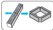
1. Remove the plastic bag from around the filter and pull the two sides of the filter apart to form a square.
