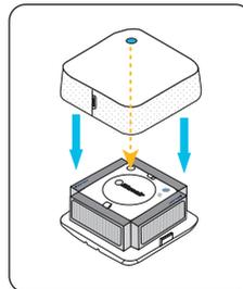
5. Remount the top cover onto the main base unit
