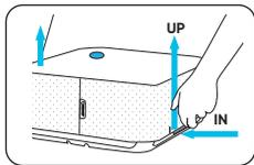
1. Place the purifier unit on a flat surface or car seat and release the top cover by pressing the left and right release locks IN and UP as shown.
