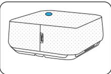
4. Turn on the unit - (a blue LED lights up on the top cover indicating the unit is powered-up).
