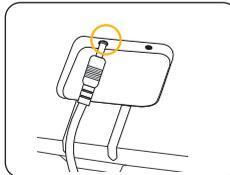
Before installing the unit into the car, connect the power cable to the power supply port on the back of the unit.
