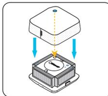
3. Remount the top cover onto the purifier base unit
