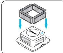
2. Mount the unfolded filter onto the purifier base unit.
