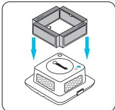
1. Lift off the top cover and mount the new filter onto the purifier base unit.
