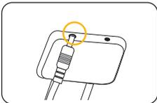
The other end of the cable is inserted into the power supply port located on the main unit.
