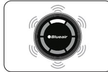
When the unit is turned on, the start up sequence begins and the fan is activated at the same speed as the last used setting. After start up the air quality is analysed and displayed on the control knob after 9 seconds.
